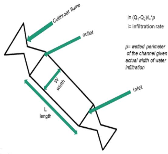
The infiltration is given by the difference of discharges between the inflow and outflow flume divided by the actual area of infiltration which is the product of length of uniform channel section and the wetted perimeter of the channel. The measurement of wetted perimeter is taken very carefully by taking average value of multiple measurements within the channel section.
