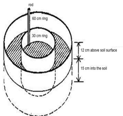
**Figure 1.** Schematic Diagram of Double Ring Infiltrometer
